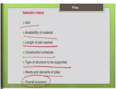
Now let us see what is the basic selection criteria for the pile, how will you select a pile? Obviously, it depends upon the type of soil, so that is why you need to do the proper geotechnical investigations to know the soil profile. So, whether it is going to be clayey terrain or it is going to
